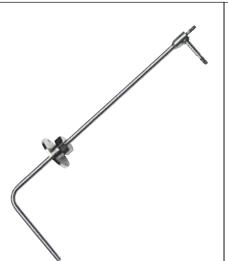
For vinyl or plastic tube (adjustable) View of "A" arrow <sup>¥</sup>R18 45 Hex.24 Static pressure hole  $\phi$  50 (multiple hole) Connector for static pressure side  $\hat{\mathbb{I}}$  $4 \times \phi 5.5$ Wind (Installation hole) Product code L (mm) "A"arrow ф 40 Total pressure hole PTTS-VT6-300-S 300 PTTS-VT6-500-S 500 (The body is made from stainless steel) PTTS-VT6-800-S 800
